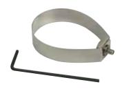
Clippard's stainless steel clamps are designed to be used with the Hall Effect and the reed switch. All clamps should be ordered based upon the size of the cylinder on which it will be mounted. The part numbers show the bore size using the numerical code. Each clamp is 3/8" wide stainless steel, and is equipped with a locking screw with #5-40 threads.
